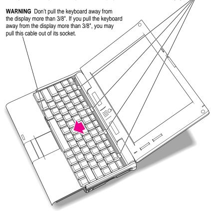
This action should release the top edge of the keyboard from its enclosure, allowing you to grasp and free the entire keyboard.
